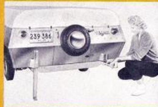
1. Adjustable levelling legs are quickly lowered and locked into position.
