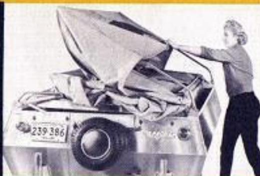
2. Traveling cover is removed and the right side of the unit is ready to be raised.
